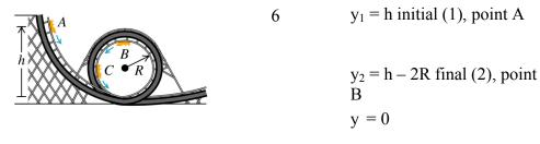
A) Find the speed of the coaster at point B. Treat the car as a particle, and assume that there is no loss of energy due to friction.  $U_{grav} = 0$
