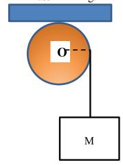
**A)** Draw a free body diagram of all the forces acting on the Box. Use Newton's law to write an equation that is a function of the tension of the rope, T, and the acceleration, a, of the box.
