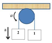
A) Use Conservation of Mechanical Energy to find the speed of Box 2 after it has fallen 0.1m. Hint: write  $I\omega^2 = \frac{I}{R^2} (R\omega)^2$ , and use the no-slip condition.
