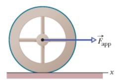
Data on wheel: mass M = 2 kg; Radius, R = 0.25 m Moment of inertia, I = 0.0625 kg•m<sup>2</sup>,
