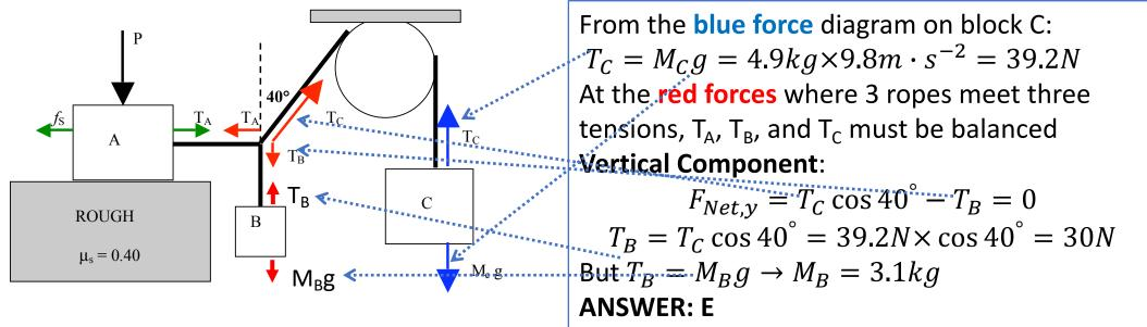
An external force P = 25.0 N is applied vertically on Block A to keep system in **equilibrium**. The mass on block B is closest to: a) 2.3 kg b) 2.6 kg c) 2.1 kg d) 2.8 kg e) 3.1 kg
