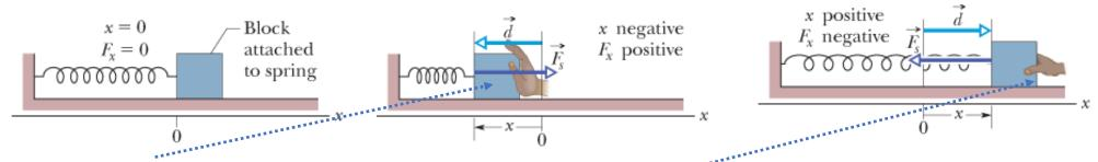
If a **leftward** force is applied to the block that **compresses** the spring, x < 0 (**left**), the spring applies a **rightward** restoring spring force,  $F_S$ :  $F_x > 0$  pushes on the block.
