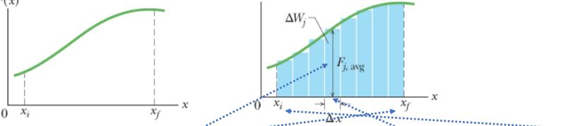
The work done is the area below the F vs. x curve from the initial position  $x_i$  to final position  $x_f$ .
